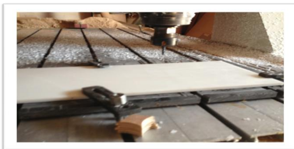
Fig. 2 Workpiece on CNC Router before machining
