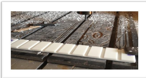
Fig. 3 Workpiece on CNC Router after machining
