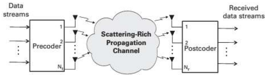
Fig 4. Generic diagram of a MIMO communication system that uses spatial multiplexing
