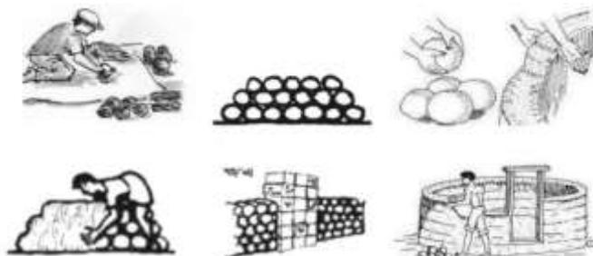
Image 5: Showing the Construction of cob
