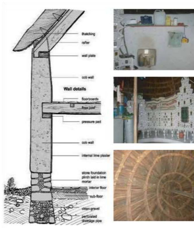
Figure 9: Typical wall section of cob wall
