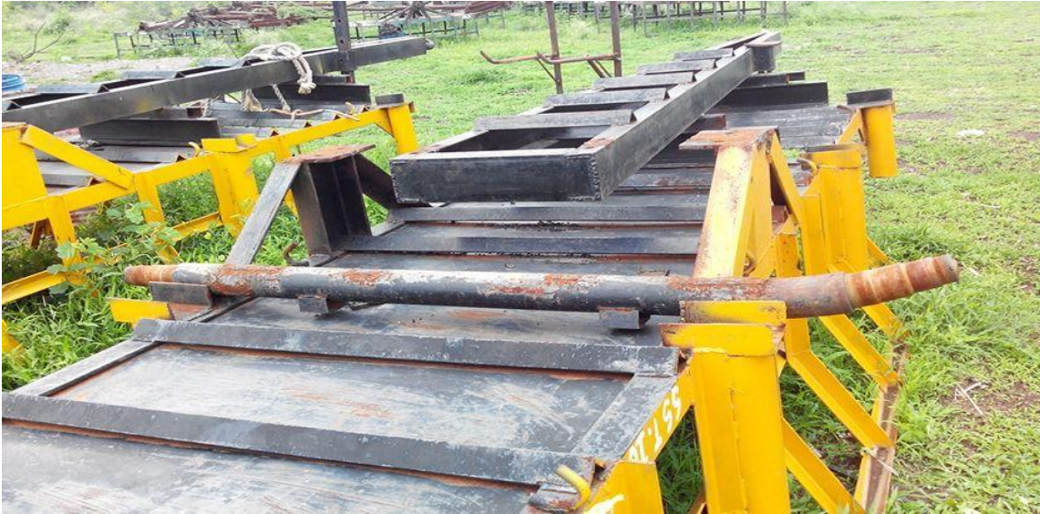
Fig. 3 Bending of sugarcane trolley axle
