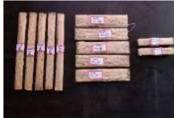
Figure.3 specimens of jute-hemp fiber-polyester resin Hybrid Composite for tensile, flexural and impact tests
