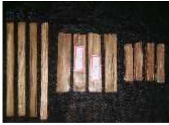
Figure.2 Specimens hemp Fiber – polyester resin for tensile, flexural and impact tests
