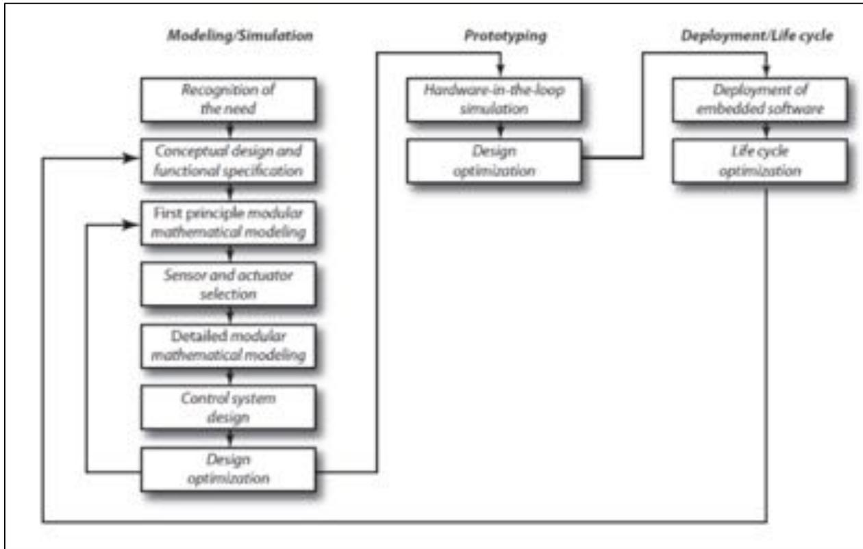
Fig 2 Mechatronic design process [10]
