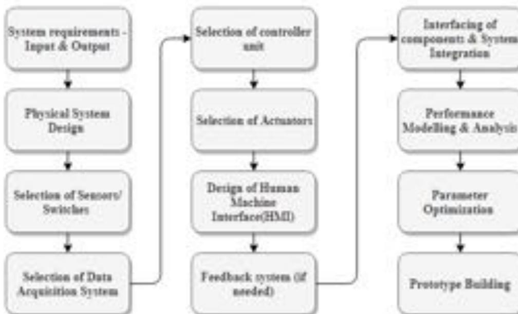
Fig: Proposed methodology for design of mechatronics system
