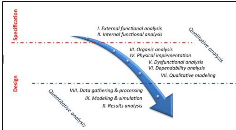
Fig: 3 Proposed overall methodology evaluating the predictive reliability of mechatronic systems [5]
