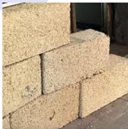
Fig.4.Precast hempcrete masonry blocks for construction.
